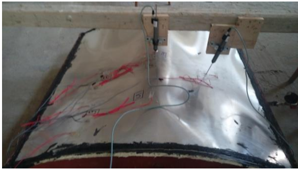
Fig. 10: Deformation shape at failure of aluminum plate
