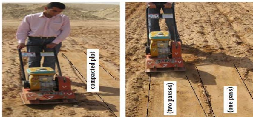
Fig. 4. Plate compactor was compacted soil during experiments
