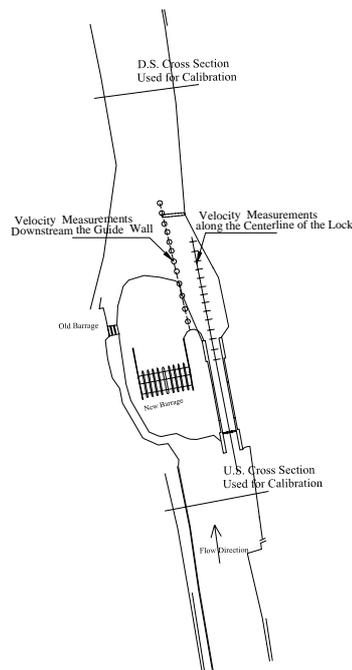
Figure 4. Cross-Sections U.S. and D.S. Saryakos Barrage used for the Model Calibration
