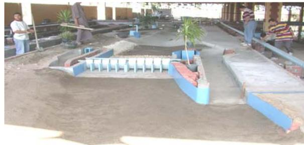
**Photo 3.** The Model after Constructing New Barrage
