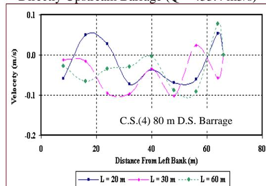
Figure 7-D. Cross Velocity Distribution 80 m Downstream Barrage ( $Q = 433.4 \text{ m}^3/\text{s}$ )
