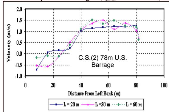
Figure 6-B. Longitudinal Velocity Distribution 78 m Upstream Barrage ( $Q_{max} = 433.4 \text{ m}^3/\text{s}$ )
