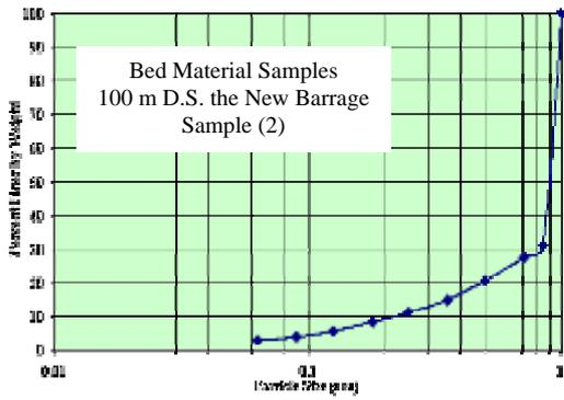
Figure 3.b. Sieve Analysis D.S. Barrage
