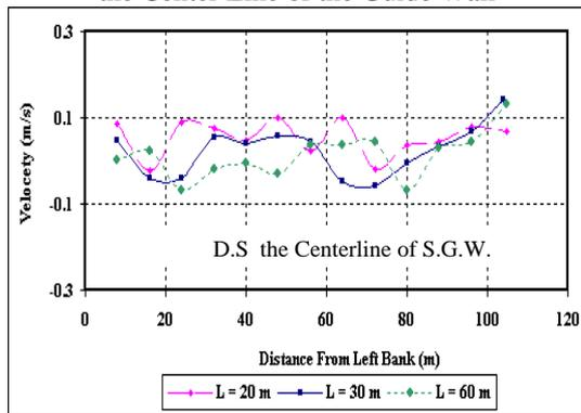
**Figure 7-G.** Cross Velocity Distribution along the Center Line of the Navigation Lock
