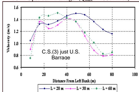
Figure 6-C. Longitudinal Velocity Distribution Directly Upstream Barrage ( $Q_{max} = 433.4 \text{ m}^3/\text{s}$ )
