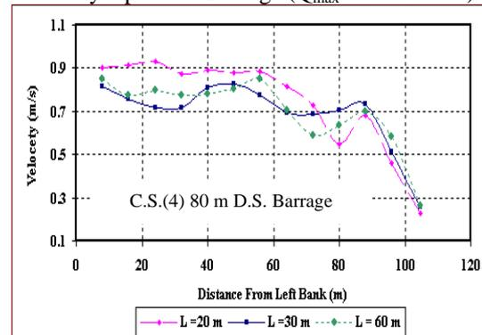
Figure 6-D. Longitudinal Velocity Distribution 80 m Downstream Barrage ( $Q_{max} = 433.4 \text{ m}^3/\text{s}$ )
