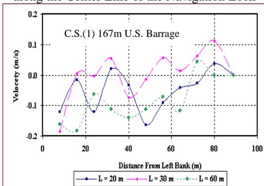
Figure 7-A. Cross Velocity Distribution 167 m Upstream Barrage ( $Q = 433.4 \text{ m}^3/\text{s}$ )
