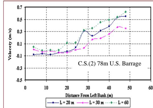
Figure 7-B. Cross Velocity Distribution 78 Upstream Barrage ( $Q = 433.4 \text{ m}^3/\text{s}$ )
