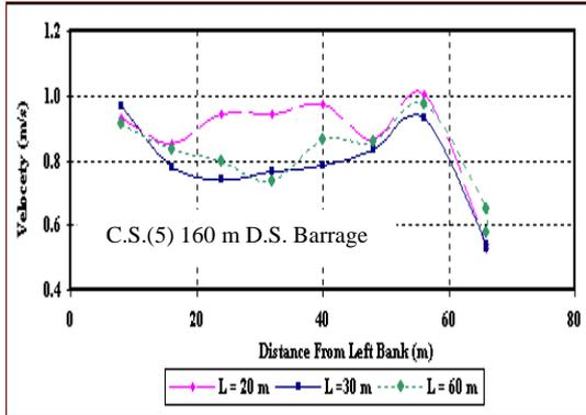
Figure 6-E. Longitudinal Velocity Distribution 160 m Downstream Barrage ( $Q_{max} = 433.4 \text{ m}^3/\text{s}$ )
