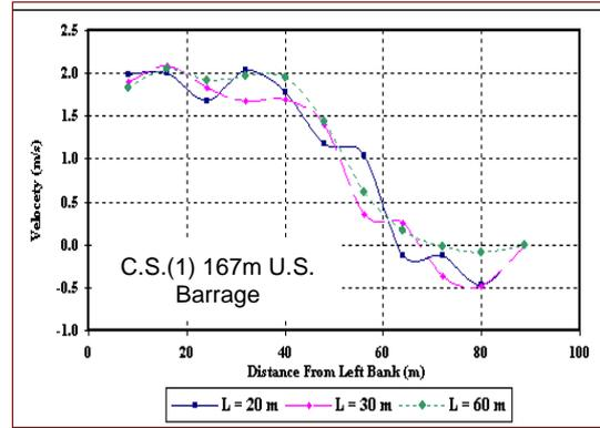
Figure 6-A. Longitudinal Velocity Distribution 167 m Upstream Barrage ( $Q_{max} = 433.4 \text{ m}^3/\text{s}$ )
