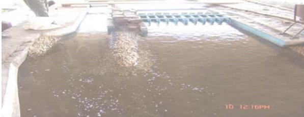
**Photo 10.** Flow Currents D.S. Barrage using 50 m Long SGW ( $Q_{min}$ )
