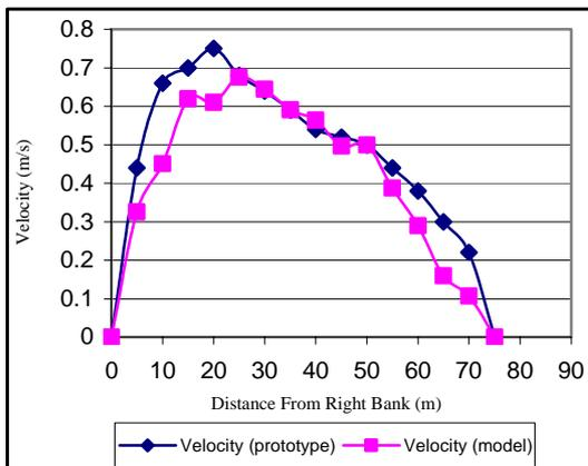
Figure 5. Prototype and Model Velocity Distribution D.S. the Lock (Calibration Process)
