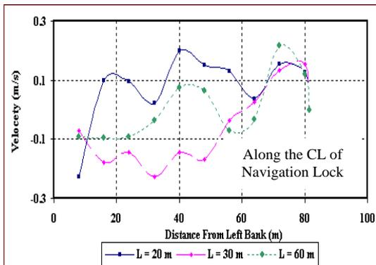
Figure 6-G. Longitudinal Velocity Distribution along the Center Line of the Navigation Lock
