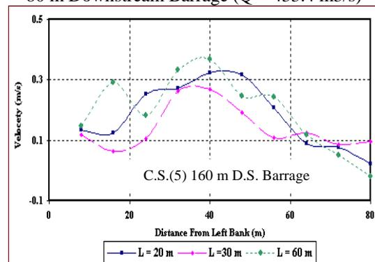
Figure 7-E. Cross Velocity Distribution 160 m Downstream Barrage ( $Q = 433.4 \text{ m}^3/\text{s}$ )
