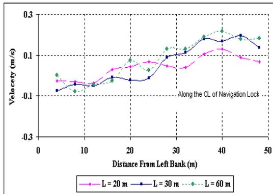
**Figure 7-F.** Cross Velocity Distribution Downstream the Center Line of the Guide Wall
