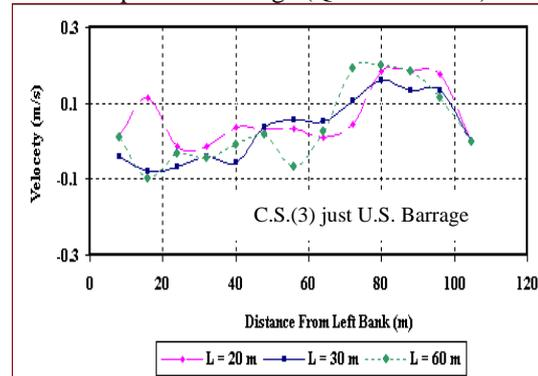
Figure 7-C. Cross Velocity Distribution Directly Upstream Barrage ( $Q = 433.4 \text{ m}^3/\text{s}$ )
