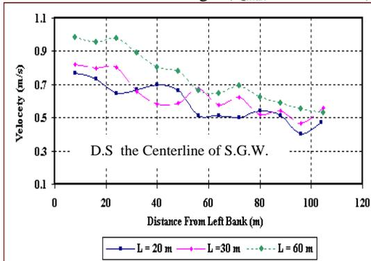
Figure 6-F. Longitudinal Velocity Distribution Downstream the Center Line of the Guide Wall
