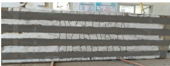
Fig. 18: Cracks pattern for S4G4L at p=160 kN
