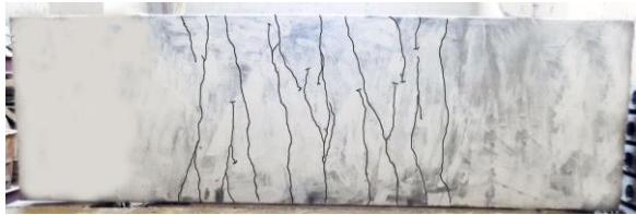
Fig. 16: Cracks pattern for CO2 at p=135 kN
