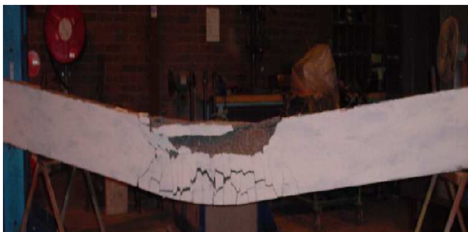
Fig. 5 Ultimate deflection for beam 12HP25
