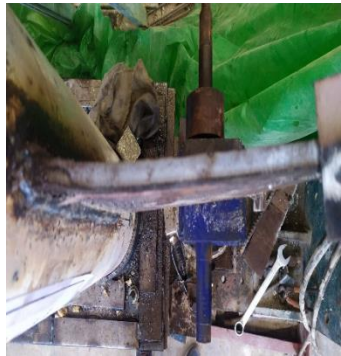
Figure 22- Deformed Shape for CWCB 6-6
