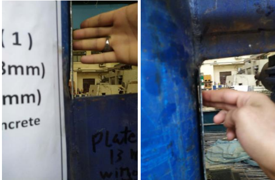
Figure 17- Description of specimen deformations for CC 6-6
