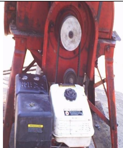
Plate 2: Diesel engine equipped with pulleys
