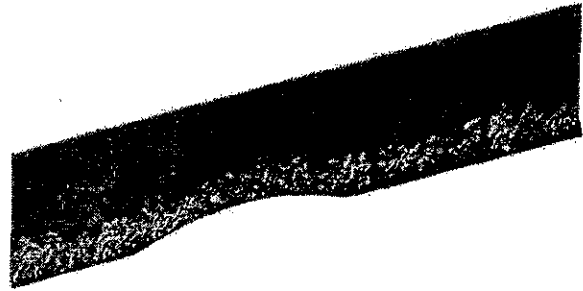
Figure 2. Iso-vorticity contours near the bump surface
