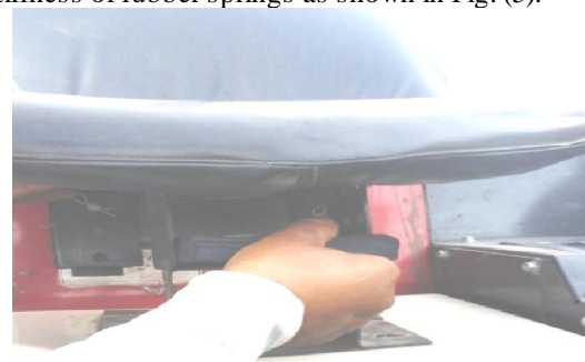
Fig. 4. Rubber spring used to reduce the rice combine harvester vibration transmitted to the operator.
