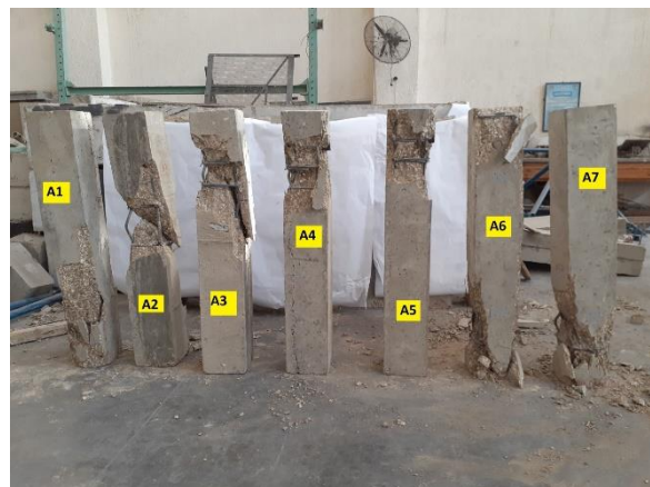
Figure 9– Failure modes of group (A) from experimental results.
