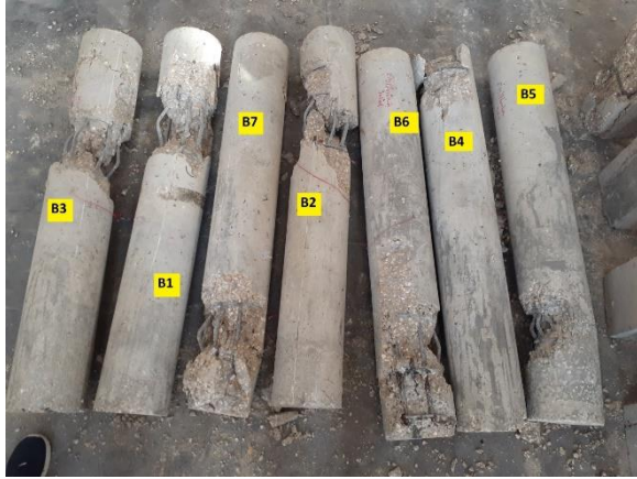
Figure 10– Failure modes of group (B) from experimental results.
