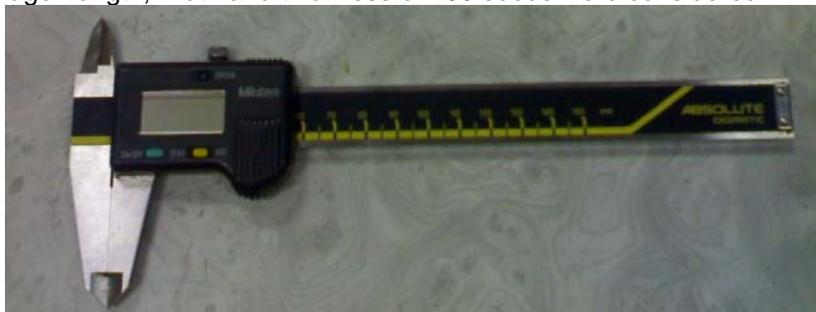
**Figure (1): Digital vernier caliber**
