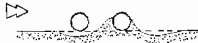
c) Scour under the first line, deposition on the second one and an attached downstream scour hole. F = 0.25, y = 2\phi, S = 2\phi
