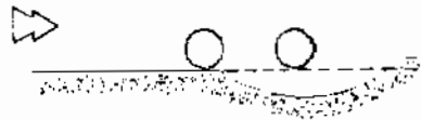
a) Scour under the second line only F = 0.285, y = 3\phi, S = 4\phi
