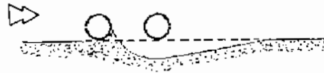
b) Scour under the second line, front erosion for the first one. F = 0.30, y = 3\phi, S = 4\phi
