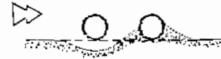
b) Scour under the first line with deposition on the second one. F = 0.19, y = 3\phi, S = 1.5\phi
